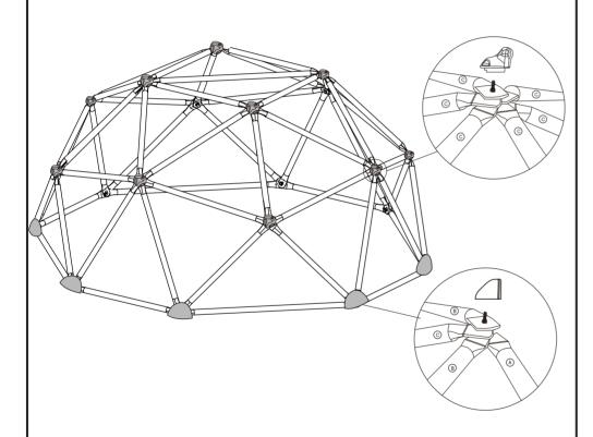
Attention: Make sure that the notch of Knob fits over the top of the tube joint.
