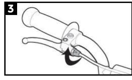
Rotate the cable adjuster barrel so the slots are aligned. Rotate the barrel adjuster to secure it.
