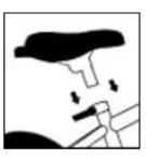
Insert seat post into frame. Adjust seat height so that the rider can touch the ground with both feet at the same time.
