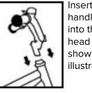
Insert the handlebar/stem into the frame head tube as shown in the illustration.
