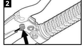
Slot the nipple end into place underneath the lever.
