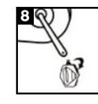
The right pedal (marked with an "R") screws on clockwise to the chain guard side crank, the left pedal (marked "L") screws on counter -clockwise to the other side.
