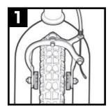
To test the function of the frog hand brake. Lift the front of The bike and spin the wheel. The wheel should not rub on the wheel. The pads should contact the rim on both sides at the same time when brake is applied. Try to move the bike and hold the brake firmly. The brake should hold well enough To keep the wheel from moving.
