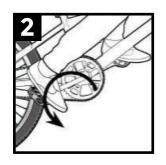
To test a coaster brake, lift the rear wheel and pedal the bicycle with your other hand. While the wheel is spinning, push the pedal backwards to engage the coaster brake. The wheel Should stop completely.
