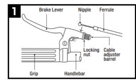
Hook-up the left-side brake lever cable that controls the front brake. Begin by loosening the locking nut on the front break. Take the loose cable on the opposite end (the end which goes into the brake lever on the handle bar).
