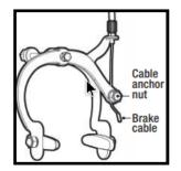
Loosen the cable anchor nut and pull the Brake cable through it. Squeeze the break Arms, pull the cable firmly through the cable Anchor nut and tighten the nut securely.
