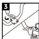
Remove the black plastic piece at the base of the handlebar, loosen the handlebar stem wedge.
