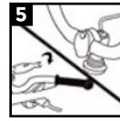
Tighten the bolt at the top of the handlebar stem.
