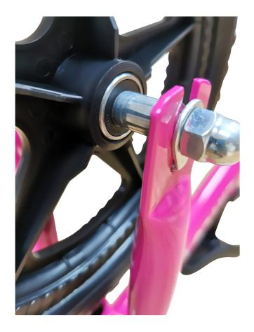
Replace the hooked washer and put into the frame hole. replace the end nut and tighten.
