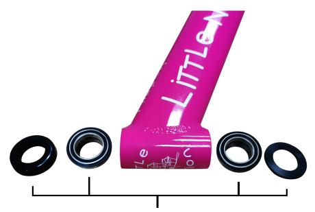
The headset consists of 4 parts. A large washer. 2 bearing bushings and a small washer. The small washer goes on the bottom of the head set and at the bas of the forks. The larger washer connects at the top of the headset.
