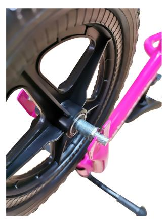
Remove the end nuts, hooked washer and long washer and push the axle through the wheel. If the axle is unable to go through the wheel. There is a washer inside the middle of the 2 wheel bearings that can me moved around by tapping the wheel.
