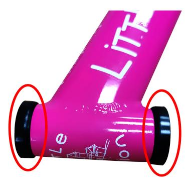
Push the 2 bearing bushings into the frame trube
