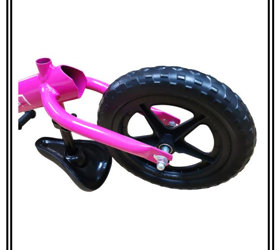
Please now go through and check all nuts, bolts and clamps have been correctly tightened
